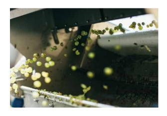
A "chroma"-function enables steplessly adjustable colour detection from the surface to the centre of objects. Further processing of the images and the easy switching on and off of sorting criteria is carried out by highly efficient microprocessors. The capacity with four cameras is approx. 5 t/h.
