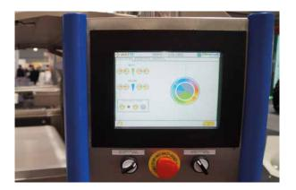
The touch screen control unit allows an easy and fast detection of desired and undesired colors of the fruit. Based on that information the setting of the color and infrared data can be adjusted. These settings can be saved in 8 memory locations.
